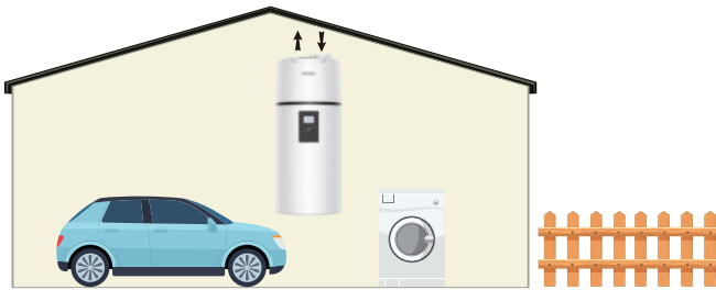
Garage or laundry room (without ducts)
