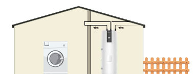
Installation with 2 ducts to the outside
